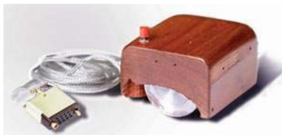
First prototype of a computer mouse as designed from Engelbart's sketches
